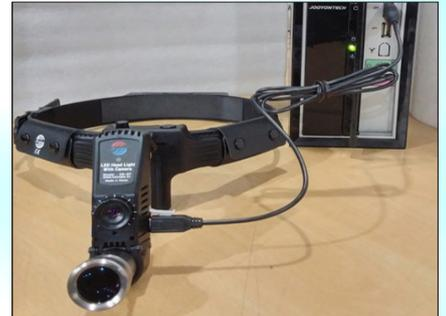
4. After turning on the headlight, after a while, when "set time complete" appear on viewer program screen, the time setting is complete.
